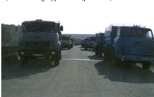
Picture 2 Loading the bridge with the test convoy
