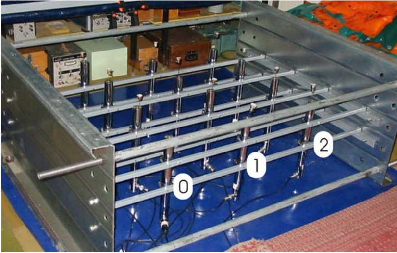
Fig.2. The testing stand with the inductive transducers
