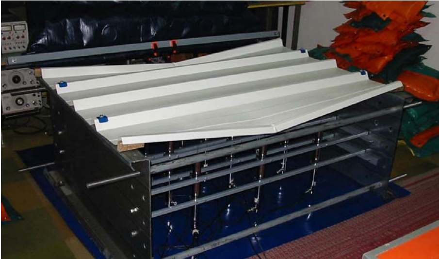
Fig. 4 The collapse of the E3-050 specimen (buckling)
