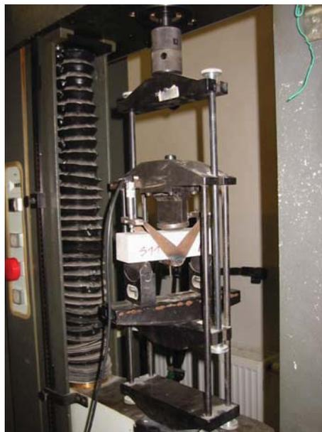
Figure 2. Three-Point-Bending-Test
