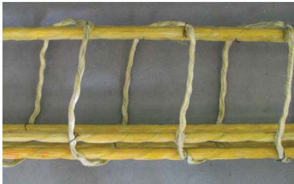
Figure 5. Shear reinforcement shaped into spiral
