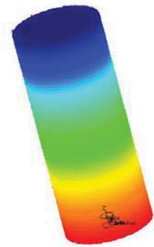
Figure 11. Longitudinal displacements (CFRP confined concrete cylinder)
