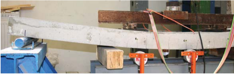
Figure 3. Deflection of the loaded beam before the collapse
