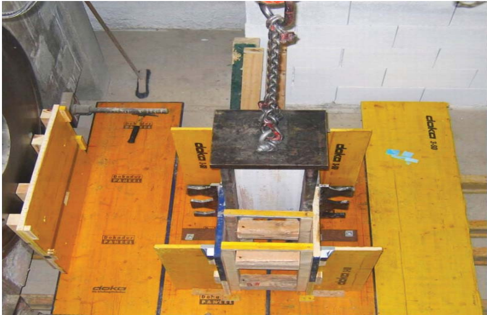
Fig. 1 Push-out specimen's welded steel parts
