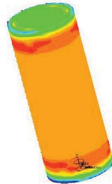
Figure 9. Normal stresses (CFRP confined concrete cylinder)
