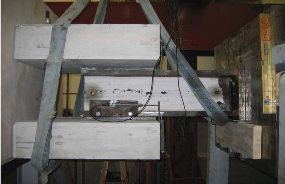
Fig. 2 Complete push-out-specimen ready for testing
