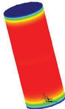
Figure 12. Transversal displacements (unconfined concrete cylinder)
