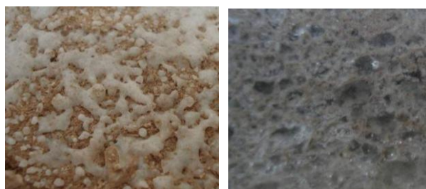
Figure 4, 5. Structure of the sample made of reference raw glass and an admixture of fluid fly-ash – FA5.0 (left) and an admixture of finely ground slag – SL5.0 (right)
