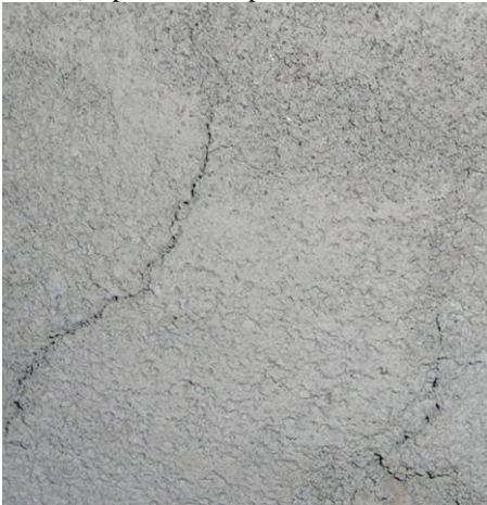
c) Specimen of plaster 1F
