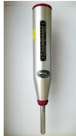
Figure 8 - Schmidt Impact Hammer type LB
