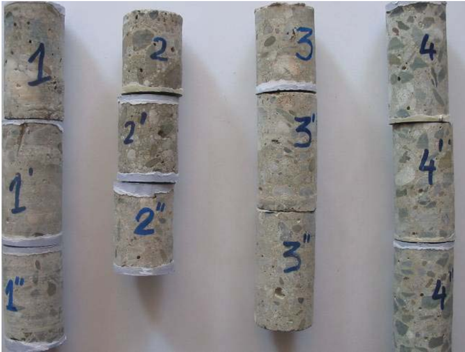
Figure 6. Concrete test rods from the superstructure
