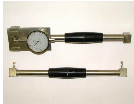
Figure 4. Dilatometer for determination of the movement of cracks
