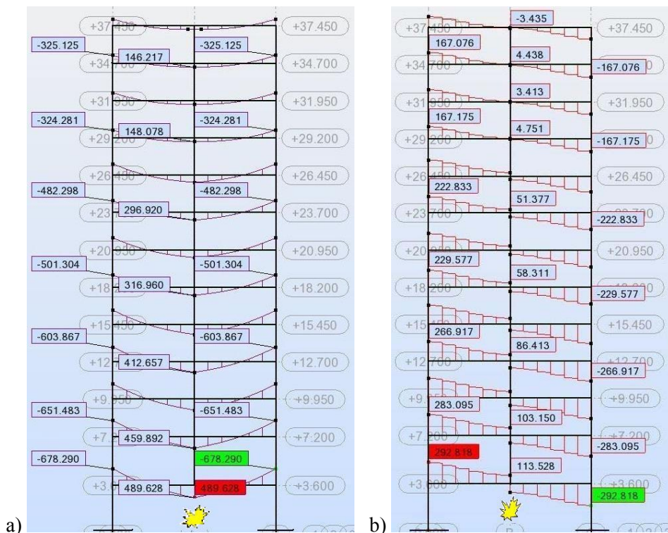
Figure 3. Damaged model P100-2006 frame CT1: a) bending moments in beams [KNm]; b) shear forces in beams [KN]
