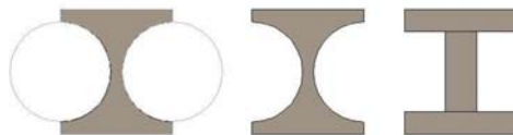
Figure 6. The equivalence of the sections of the concrete slab with spherical gaps
