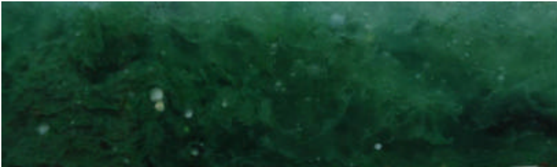
Figure 7. Capturing the structure of a sample made of car glued glass at the maximum temperature of 1050 °C, with the addition of 0.7% of green pigment.
