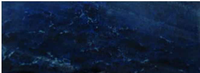
Figure 5. Capturing the structure of a sample made of TV monitor cullets at the maximum temperature of 900 °C, with the addition of 1.2% of blue pigment.
