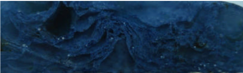
Figure 8. Capturing the structure of a sample made of car glued glass at the maximum temperature of 980 °C, with the addition of 0.5% of blue pigment.
