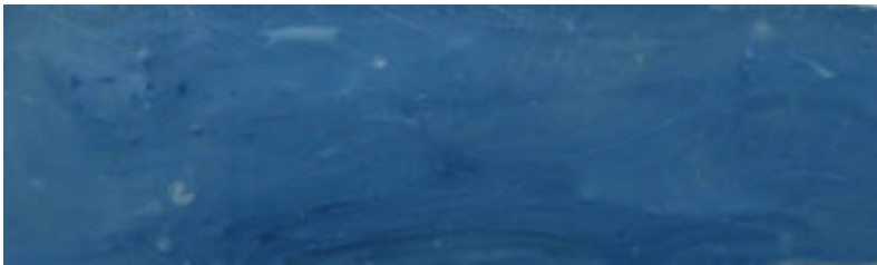
Figure 11. Capturing the structure of a sample made with using the cullets of linear fluorescent lamps at the maximum temperature of 820 °C, with the addition of 0.5% of blue pigment.
