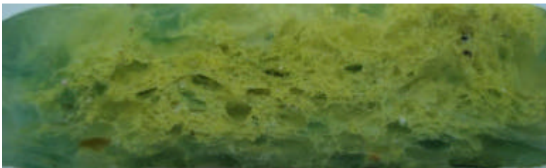
Figure 9. Capturing the structure of a sample made of car glued glass at the maximum temperature of 980 °C, with the addition of 1.5% of yellow pigment.
