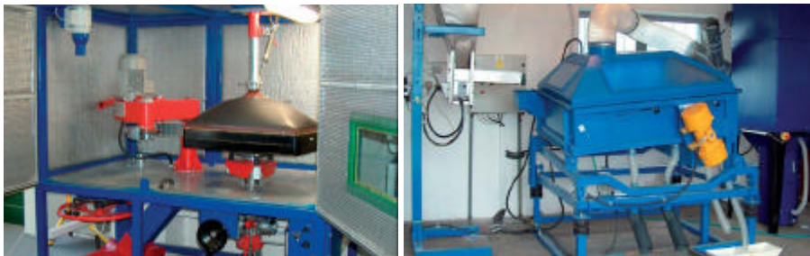
Figure 1. Line intended for separating various parts of the TV-monitor glass (on the left), technological equipment intended for removing luminophor from the CRT monitor (on the right) [2]
