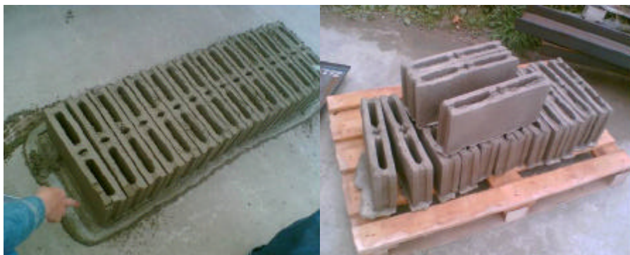
Figure 2. Initial design. Too plastic mortar after vibropressing
