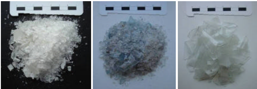
Figure 1. Recycled cullet used, from the left side - glass coming from recycling the TV monitors cones (CR), recycled piece of front car windshield (AG), glass of fluorescent lamp (FT)
