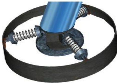
Figure 6. Base isolating system
