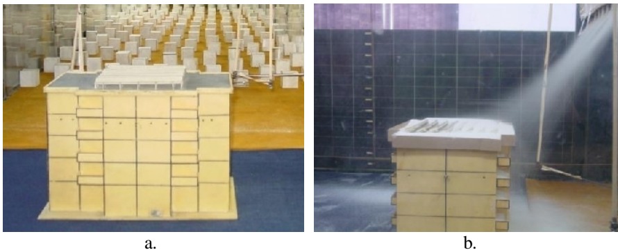
Figure 6. Experiments in SECO2 wind tunnel: a.- the model of the building with solar panels, b.- simulation of blizzards
